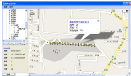
Figure 21. Abnormal operation of streetlight in nighttime
