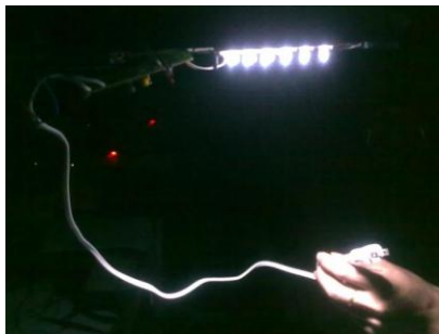
Figure 17. Normal operation of LED light during a power outage
